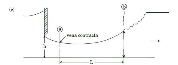
Consider a vertical sluice gate in a wide rectangular channel. The depth of flow at the vena contracta is 0.457 m for a flow rate of 4.646 m<sup>3</sup>/s per metre of width. The channel bed slope is 0.0003 and Manning's roughness factor is n = 0.020. The depth of flow at point b is 0.5 m.
